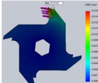
Gambar 15. *Displacement* Pada ASTM A36 dan HSS 18%
