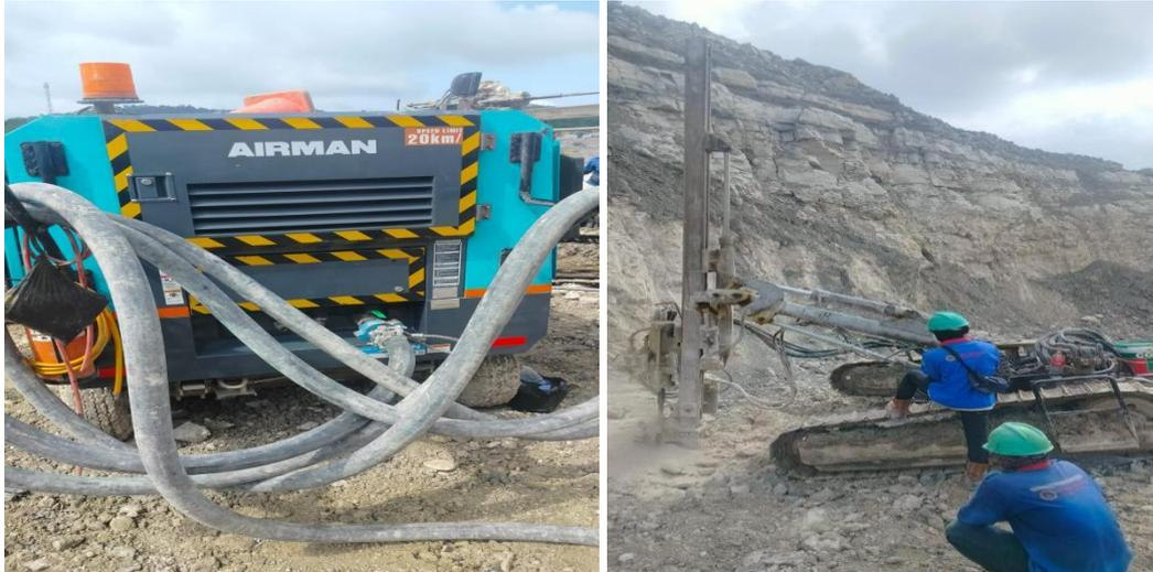
**Gambar 1. Compressor Airmann PDS750S & Crawler Rock Drill Furukawa PCR 200**
