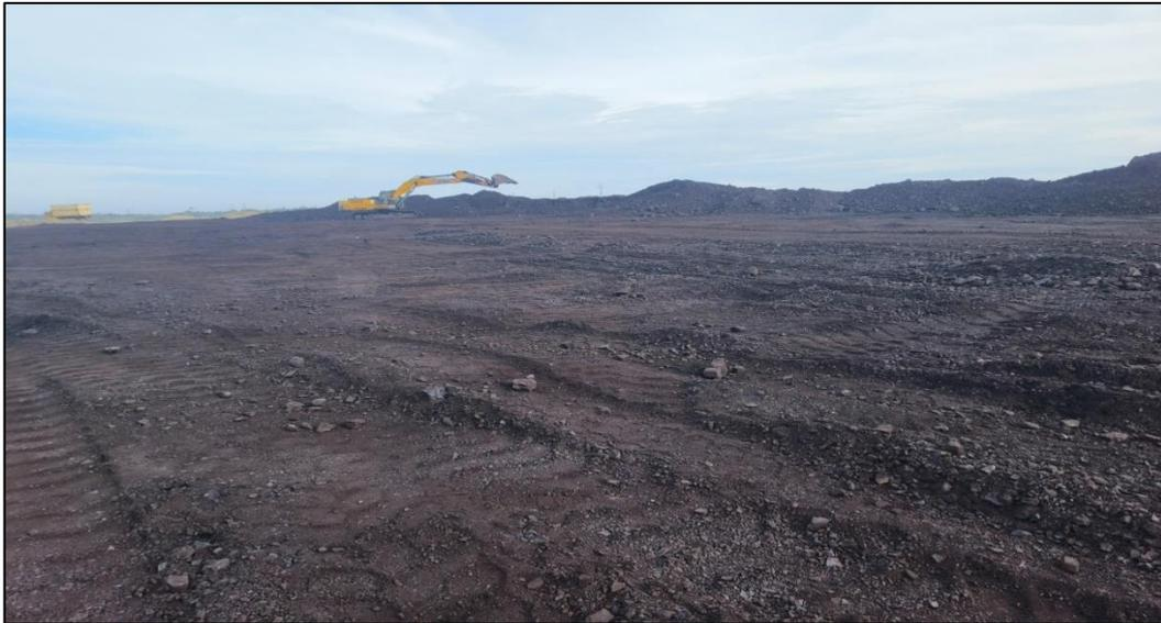
**Gambar 4. Bedding Coal di ROM Stockpile**
